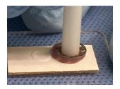
• Finally, the wider end of the assembly tool is used to press the back plate firmly down into the groove, usually with an audible sound. The assembly tool must be perpendicular to the front plate when pressing down.
